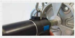
Special accessories: **Angular adapter** to maintain the necessary perpendicularity to the part.
