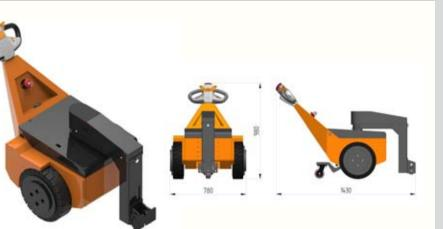
Wheels and Tyres Drive Wheel: Solid black rubber Rear Castor: Polyurethane castor
