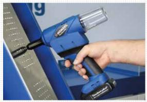
ALL IN ONE. THE VARIO NOSEPIECE For quick and easy changing between the diameters 2.4 mm, 3.0/3.2 mm, 4.0 mm and 4.8/5.0 mm - completely without tools (special accessory)!
