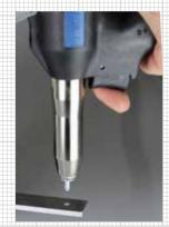
Flat standard nosepieces with reduced dog point improve the setting behaviour and make the work process faster.
